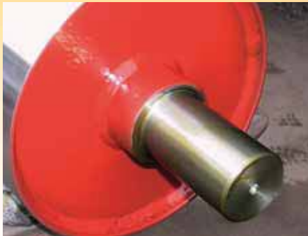
e.g. shaft welded
