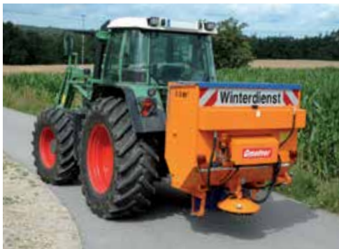
Fig. 6: Level control or road salt
