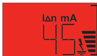
Figure 17:Leakage with prealarm screen
