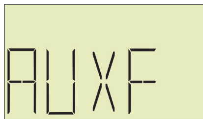
Figure 13: Fault relay screen.
