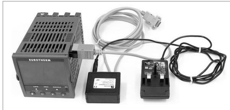
The Ethernet and DeviceNet communications module should not be fitted while using the CFG Clip as communications conflicts will occur. This is because both the DeviceNet and Ethernet Communications Modules maintain constant messaging between themselves and the instrument even when no external messages are being received.
