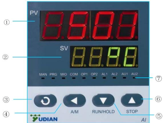
⑦ Indicator lamps: OP1 and OP2 indicate the status of current retransmission. AL1, AL2, AU1 and AU2 indicate the I/O actions of the corresponding modules.
